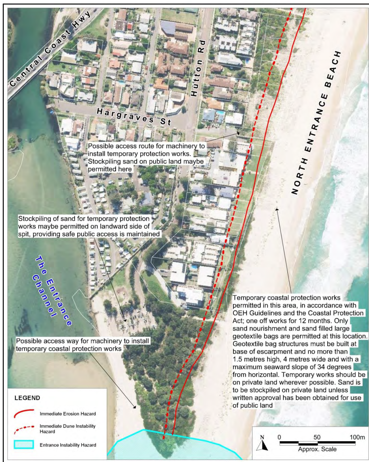
Figure 2-1 Temporary Coastal Protection Works Options for Private Property at North Entrance Beach – Hutton Road
